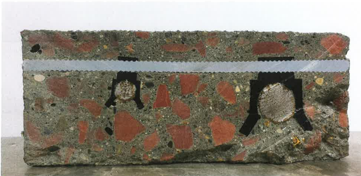
Fig. 2: Section of consolidation of concrete around side form spacer assembly using plastic coil rod.
