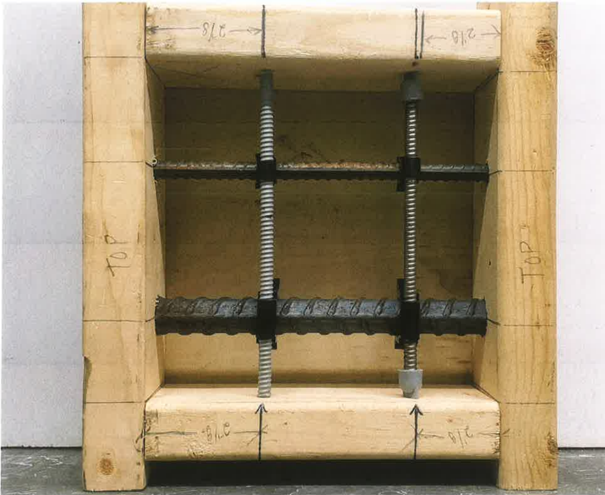
Fig. 1: Above show the aggregate flow test form preassembled by Mr. Michael Rush
