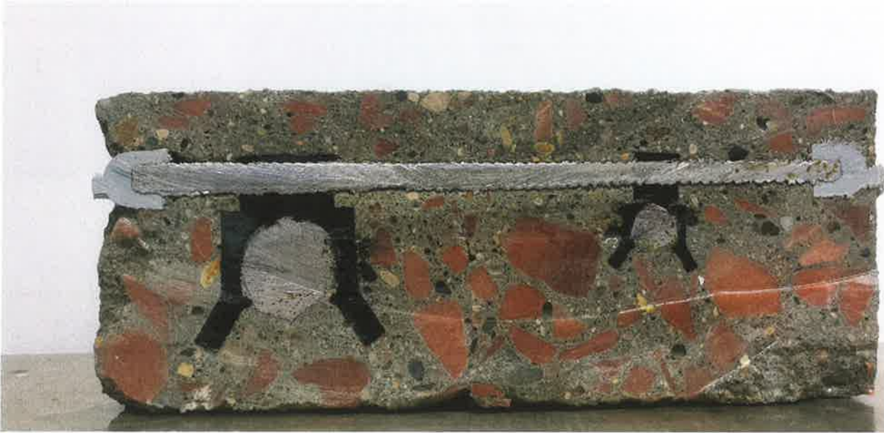
Fig. 3: Section of consolidation of concrete around side form spacer assembly using metal coil rod and plastic end caps.
